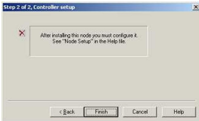
After a moment, you will see a notice telling you that after installing this node you must configure it. What you are actually doing is preparing the flash memory to accept the programming information from AccessBase. One of the steps in the process is to erase the flash memory.
